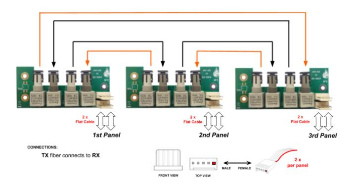
The following image shows a single wiring connection, normally used for CHAMELEON Display extension or BMS connection.
